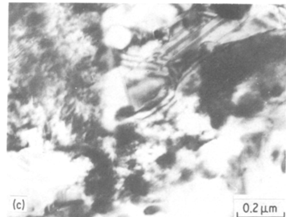
Figure 4 Transmission electron micrographs of Co-3% Ti alloy deformed 40% and subsequently aged at 873 K. (a) As-deformed: showing high density of dislocations and their distribution. (b) After 0.5h: showing heterogeneous precipitation in the recrystallized region and dislocations. (c) After 3h: showing increased precipitation in the recrystallized region and un-recrystallized region with dislocations.
